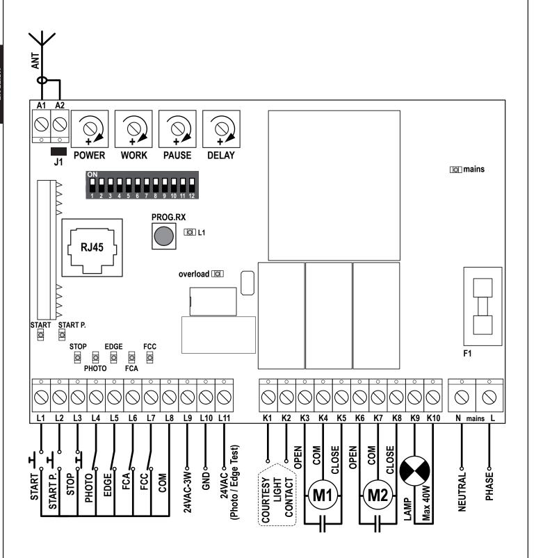
PLEASE NOTE: If not used, the normally closed inputs (STOP, PHOTO, EDGE, FCA, FCC) must be jumpered with the commands common line COM (-)
